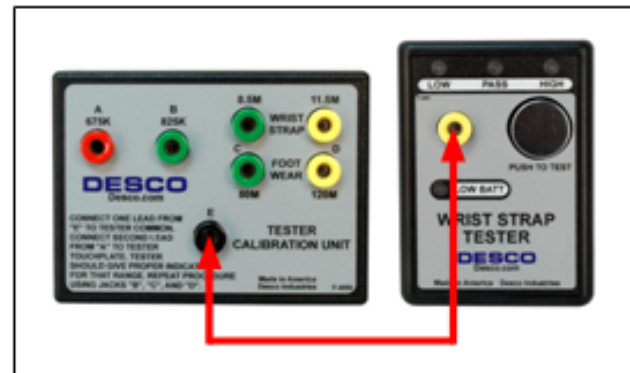
Figure 2. Connecting the test lead from banana jack "E" on the Calibration Unit to the banana jack on the Wrist Strap Tester
