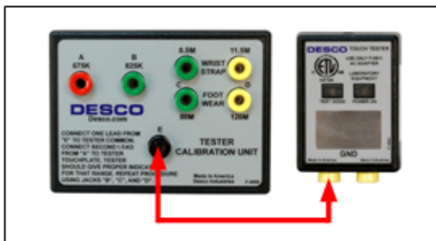
Figure 8. Connecting the test lead from banana jack "E" on the Calibration Unit to one of the banana jacks on the Wrist Strap Touch Tester
