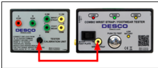
Figure 4. Connecting the test lead from banana jack "E" on the Calibration Unit to the WRIST STRAP banana jack on the Combo Tester
