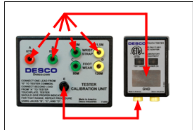
Figure 9. Verifying the calibration of the Wrist Strap Touch Tester
